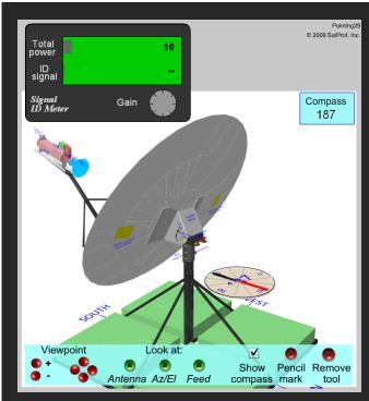
The full 3-D interactive antenna simulator, with operating meter and compass, teaches antenna pointing and evaluates real-world pointing skill.
